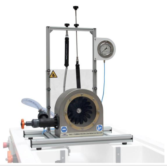
The TH.01.1 equipment simulates an instalation in a small scale with a Pelton turbine. It has been designed with special emphasis on the didactic aspect of the same, being able to observe at all times the operation of the system and the different components that constitute it.
