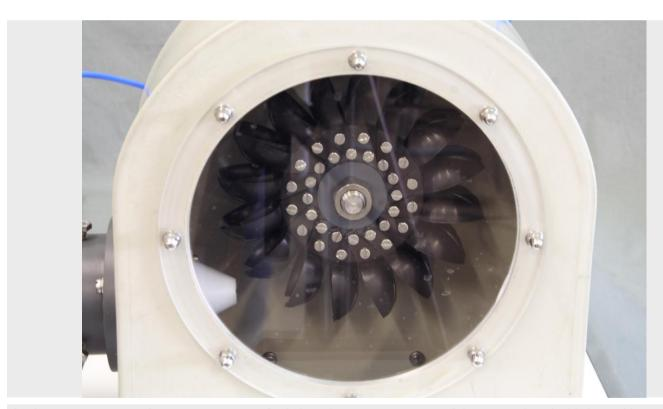
Thanks to its transparent front, you can see perfectly how the water coming out of the injector hits the blades and how, depending on the speed of rotation, the moment the water leaves the blade, in function of the relative velocity of the water relative to that of the impeller.
